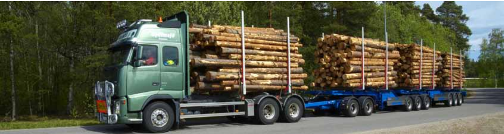
The ETT project (Modular system for timber haulage) is a Swedish project involving a trial of a timber truck that can carry four stacks instead of three, resulting in a reduction in diesel consumption, carbon emissions, road wear and transportation costs.
