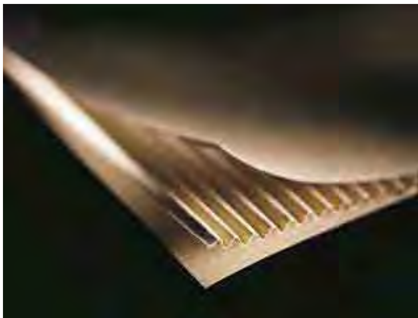
Cross-section of corrugated board showing the middle layer, fluting, encased in the outer layers, liner.
